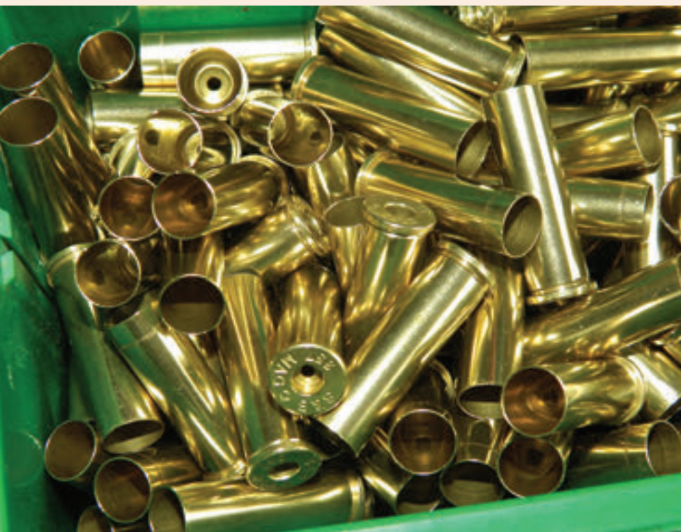
Lyman Cyclone does a great job of cleaning and polishing inside, outside, and primer pockets of cases, as shown here with this batch of .357 Magnum.
