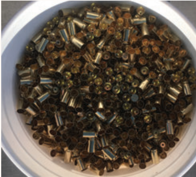
Tumbling approximately 6,000 pieces of .45 cases in Lyman Cyclone was accomplished in a fraction of the time it would have taken in a vibratory tumbler.
