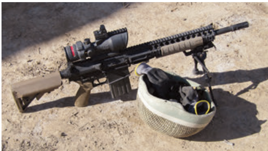
Brit LMT with its issue six-power ACOG on patrol halt in Afghanistan. As pictured, marksman's rifle dresses out at about 14.5 pounds.
