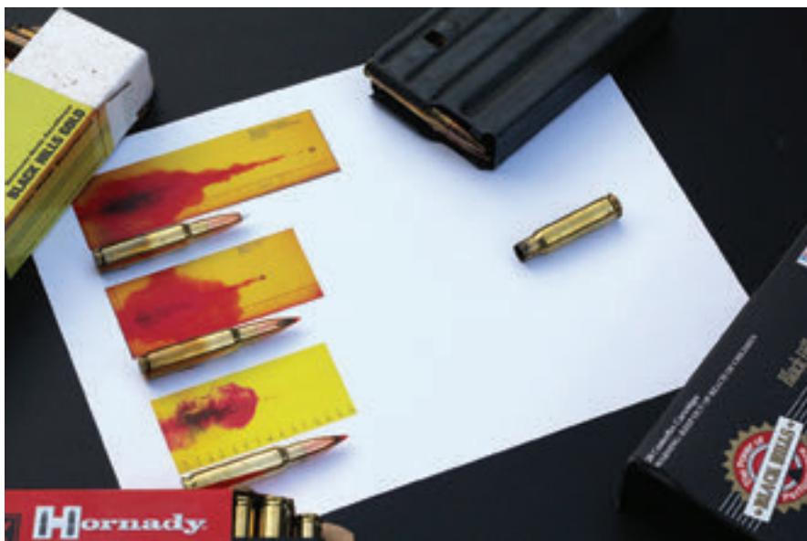
Strong suit of 7.62 is versatility in load selection. Top to bottom: 180-grain Black Hills Accubond, 155-grain Black Hills AMAX, and 110-grain Hornady TAP, alongside their ballistic gel penetration.
