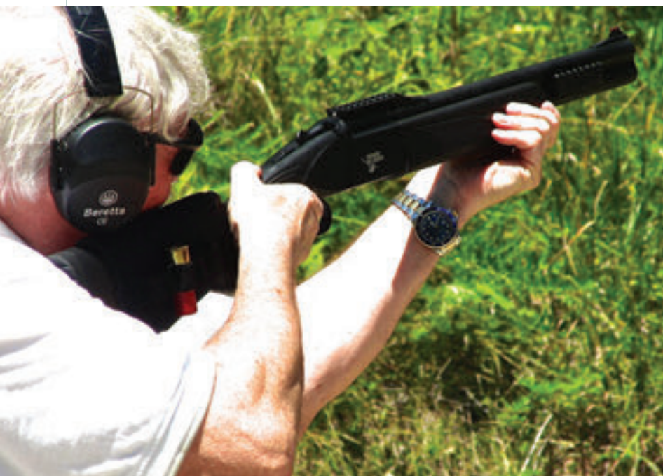
Muzzle flip when firing Federal Tactical 00 Buckshot. Because Mossberg HS12 TR is light and compact, recoil is more apparent than with most combat shotguns.
