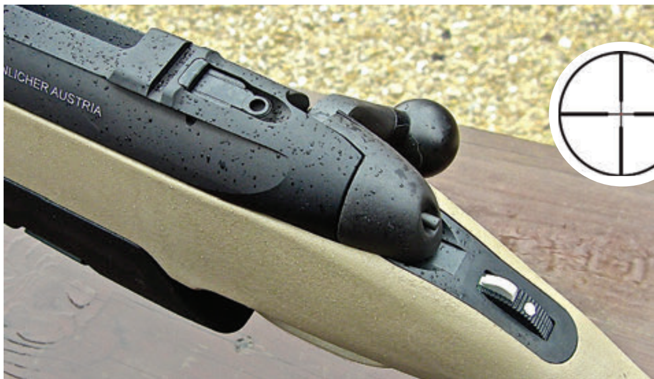
Scout Tactical's features include folding back-up rear sight, good-sized bolt knob for fast operation, protruding pin indicator that rifle is cocked, and roller safety on safe. Inset: Leupold FireDot Duplex reticle for 1.5-5X33 VX-R Scout Scope.
