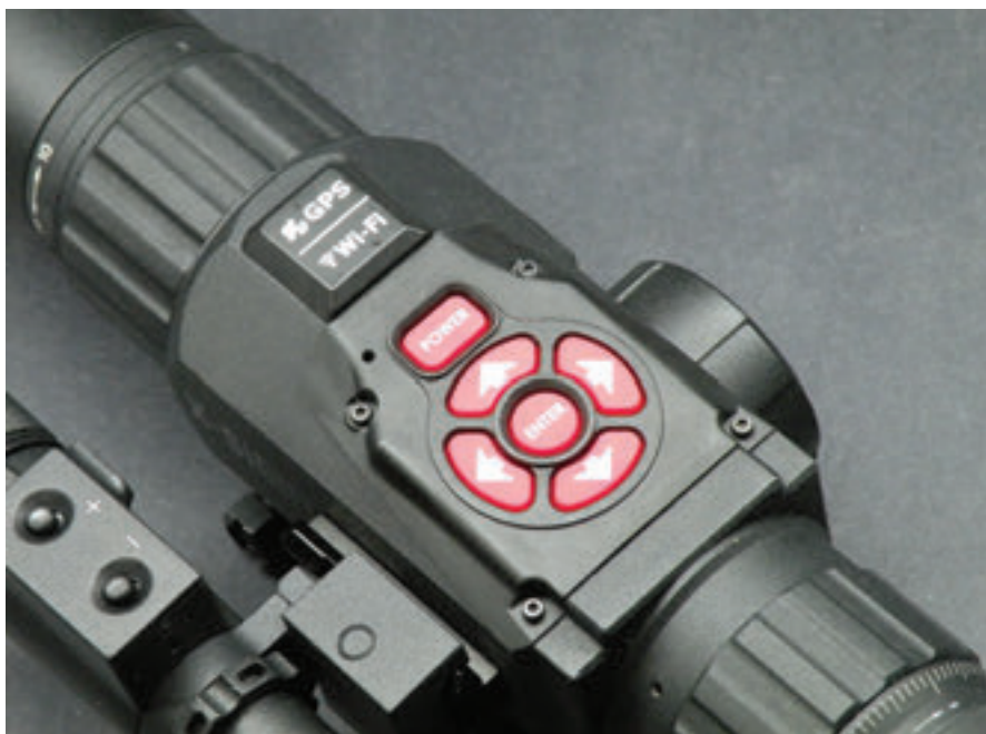
Top view of X-Sight shows control panel for this new digital day/night scope.
