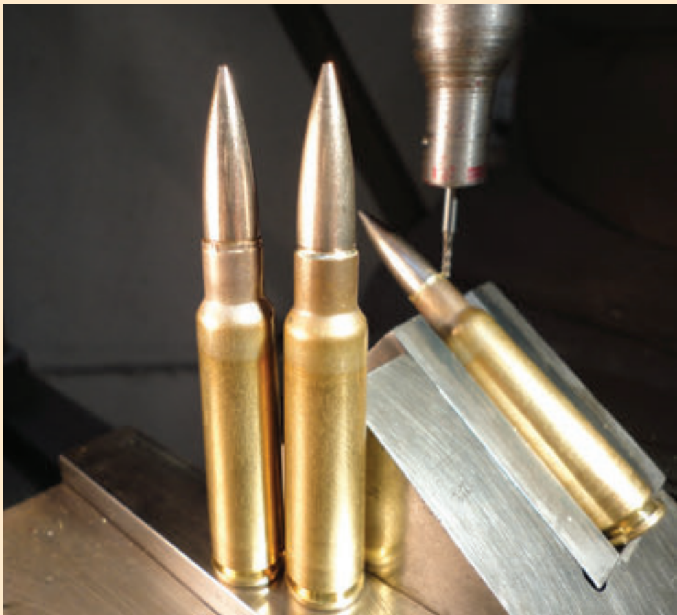
Round on right has had the crimp removed in an unsuccessful attempt to remedy fliers.
