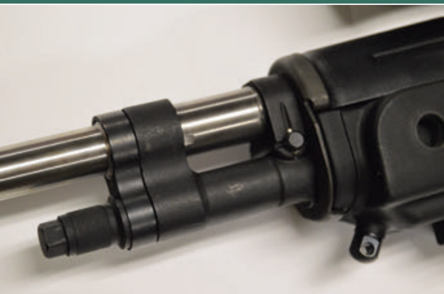
Gas system on accurized M1A is a fitted unit to get consistent gas flow through the gun, translating to greater consistency in gun's cycle of operation.
