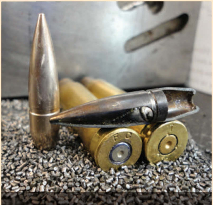
Swiss GP11 (1992 manufacture in this case) ammo comprises a spire-point 174-grain FMJ boat tail with thickish plated steel jacket, Berdan primed case, and 51 grains of powder. Sectioned bullet has lead core melted out; 7.5 case (right) is .023 inch larger in diameter and 3/16 inch longer than .308 case (left), and approaches .30-06 case capacity.
