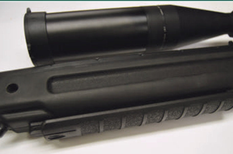
Forend has a rail system mounted underneath (here with cover on) to attach various accessories or bipods. Bipods can also be attached to bipod stud at front of forend.
