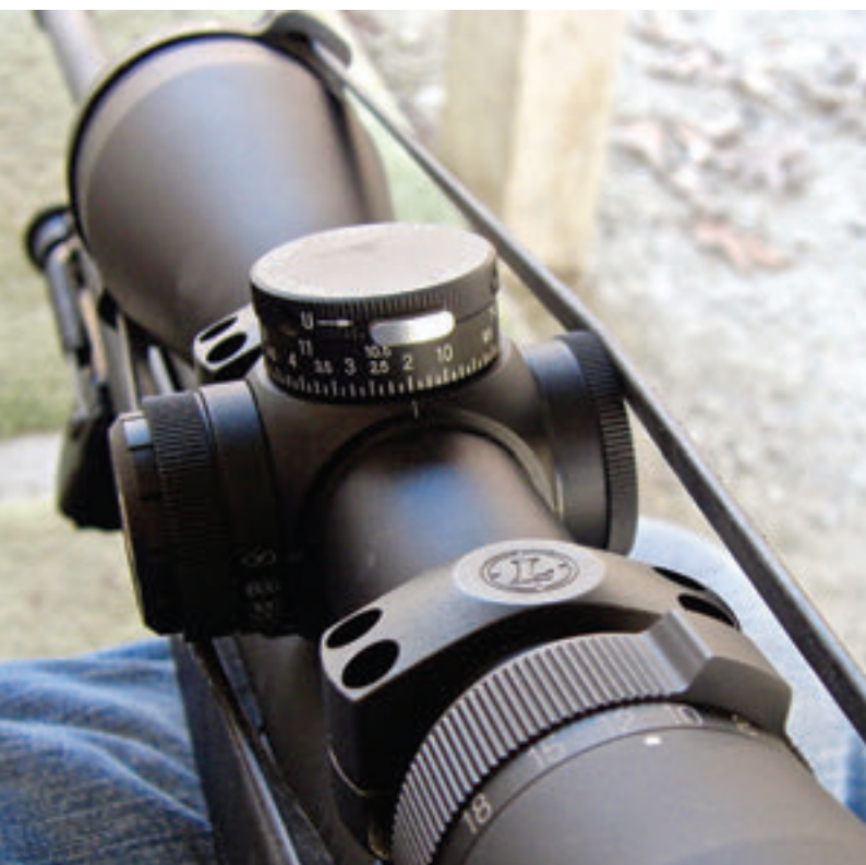
Elevation dial zeroed to 200 yards. Also note zero-lock button above the "2."
