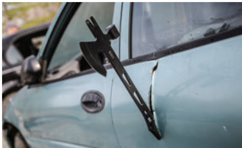
Metal cutting claw on VTAC Operator Axe makes quick work of cutting auto and aircraft sheet-metal panels. Photo: 5.11 Tactical
