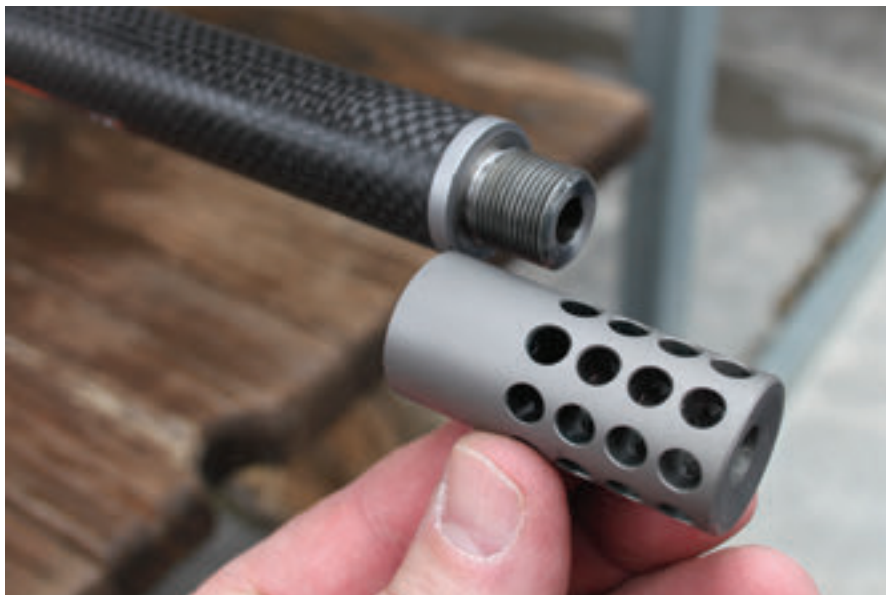
Above: Radial titanium muzzle brake is threaded on the Match carbon-fiber wrapped barrel via 5/8x28 threads.
