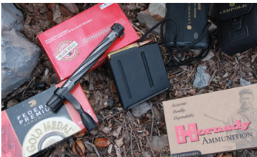
Below: Fluted bolt is Nitride coated at 70 HRC for extreme wear protection. Rifle is fed via five-round detachable magazine. Leupold RX-1200i laser rangefinder supported field testing.
