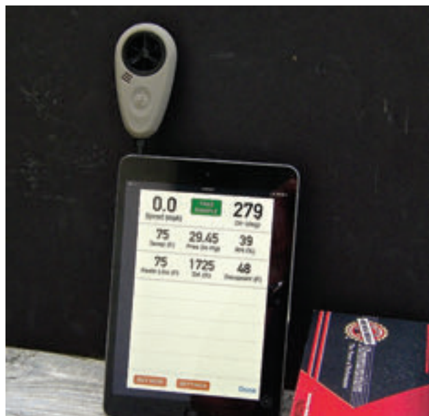
Above: Target solution from BallisticsARC and WeatherMeter shows adjustments for elevation and windage. No windage adjustment was necessary for this shot. Right: WeatherMeter plugged into iPad for hands-free taking of data.
