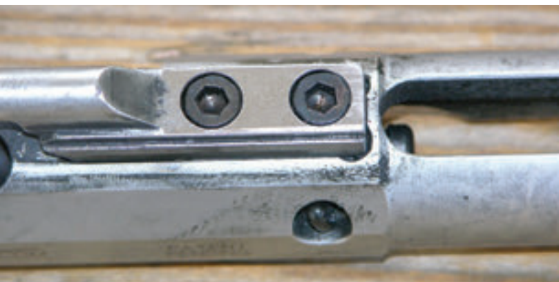
Above: This bolt carrier key has not been staked.
