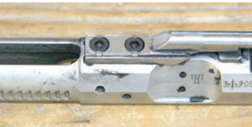
Below: Keys are properly staked. Entire elapsed time is about a minute and a half. Ever wonder why some makers don't do this at the factory?
