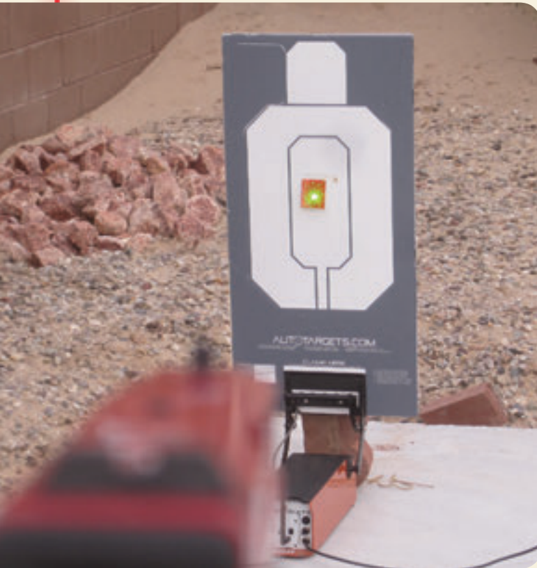
Reflective tape allows SIRT Pistol to be used in bright daylight.
