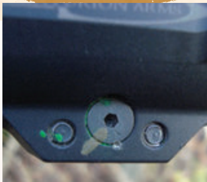
Centurion rail attachment is as good as any, but screws like to come loose. Author staked the three clamping screws for added security.
