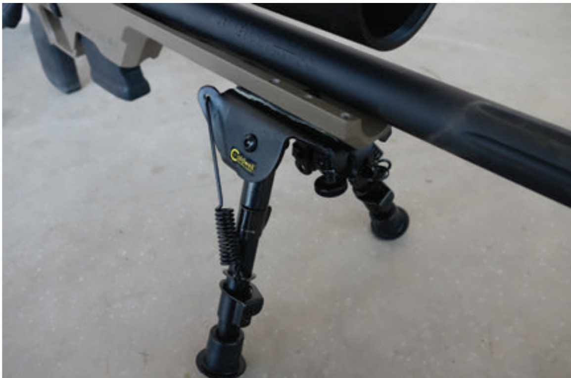
Sixteen-inch barrel is free-floated in skeleton chassis. Bipod comes standard from the factory.
