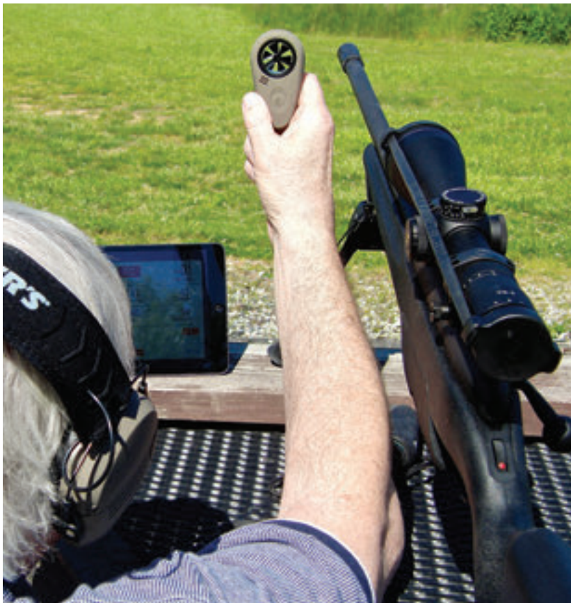
WeatherMeter can be plugged into a mobile device to gather info hands free, but Thompson prefers holding it in the air to catch the wind better.
