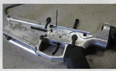
Above: Bolt release is held in a bit differently than .223 AR: pin is held in by a tiny screw. This allows operator to adjust tension.
