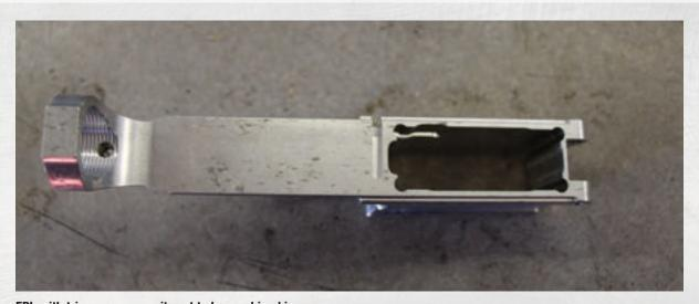
EPL with trigger group cavity yet to be machined in.
