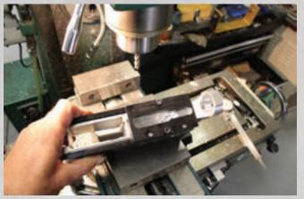
Above: First part of cavity finished, with jig for shelf in place. Depth for shelf is .525 inch.
