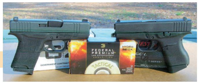
Bowie custom G43 (left) and stock G43. Custom G43 has grip reduction and stippling, rounded trigger guard, magazine removal cutouts, and slide treatment.
