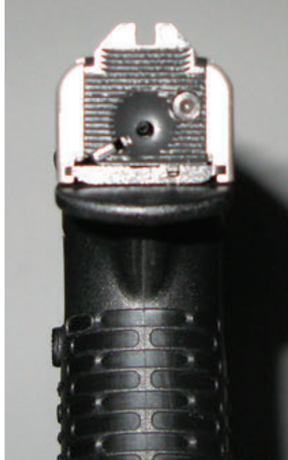
Back plate with rear sight aperture indicates striker is cocked.
