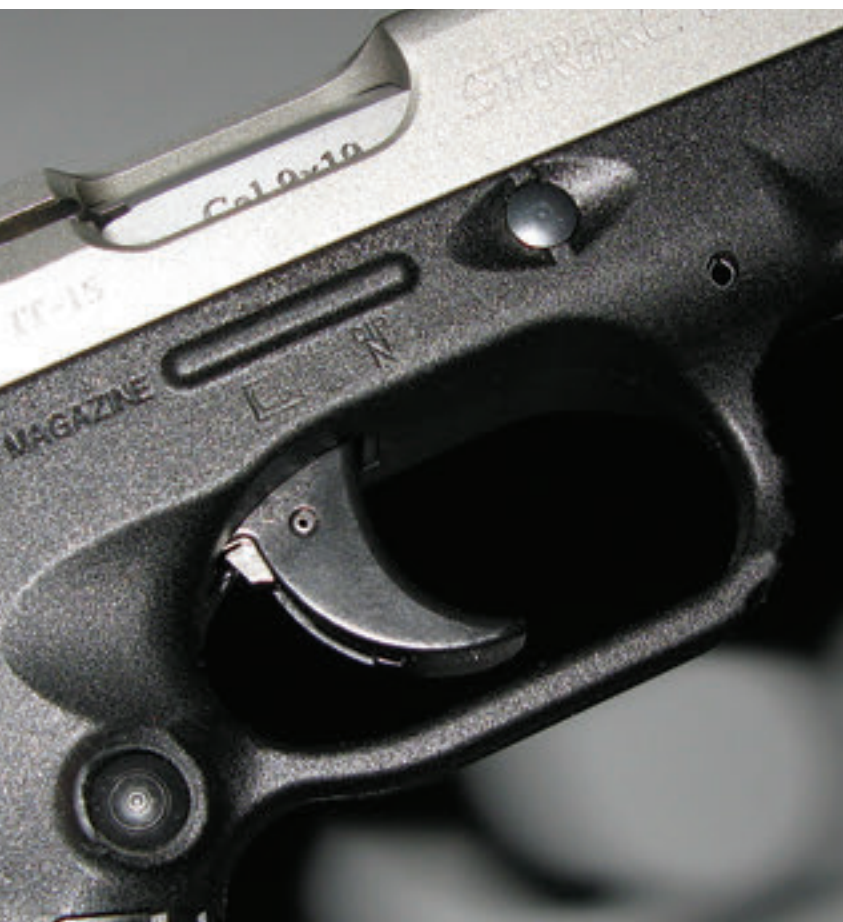
Four-pound two-stage trigger is relatively smooth with a crisp break. Reset is rather vague. Note stainless trigger safety behind trigger. Pin below slide is takedown pin.
