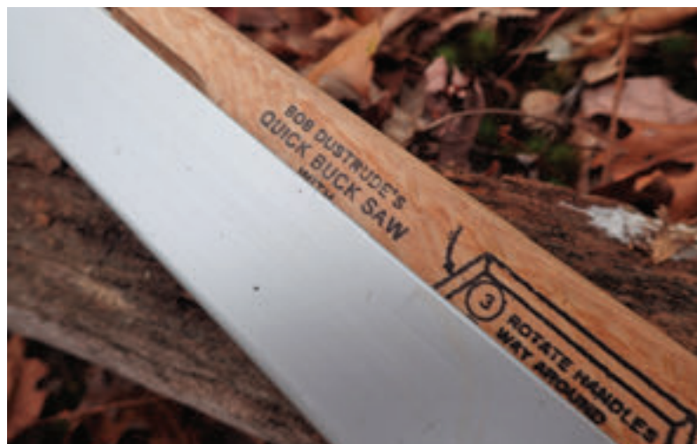
Above: Heavy-duty folding buck saws designed and handcrafted by Bob Dustrude in northern Minnesota. The 21-inch saw weighs only 15 ounces.
