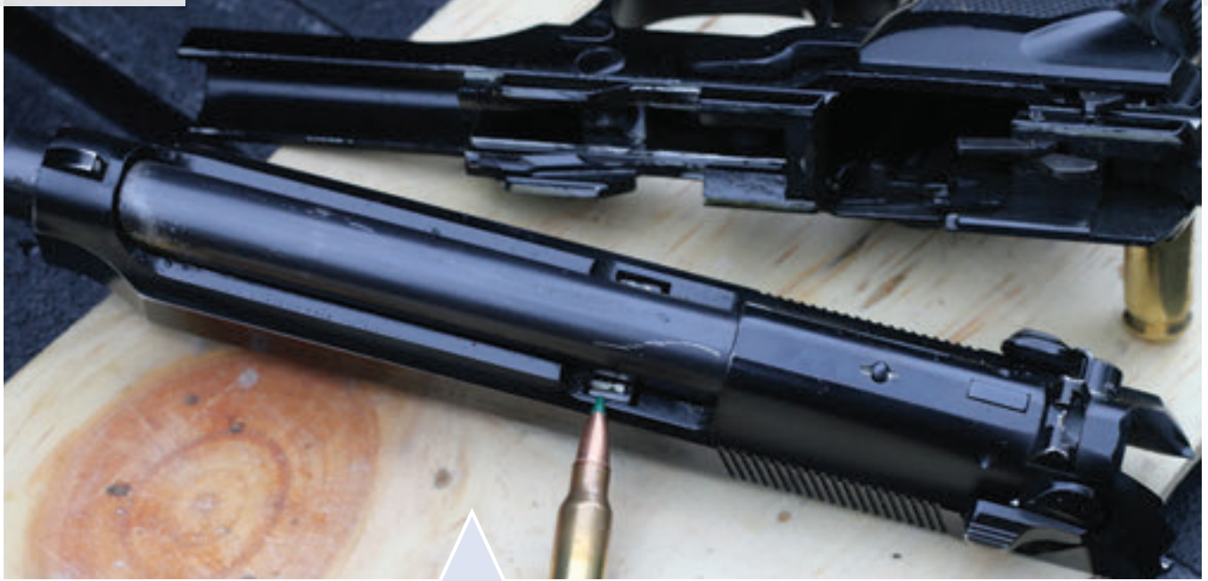
M9 gets best use of lube applied to each lug of the locking block.
