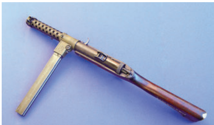
Above: Right side of Lanchester shows brass buttplate, magazine housing, and safety notch into which bolt can be rotated.
