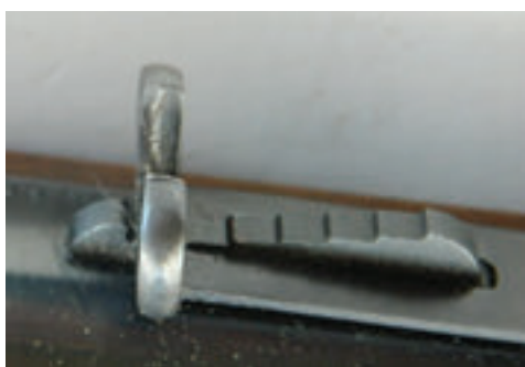
Left: Rear sight is adjustable via a sliding ladder.
