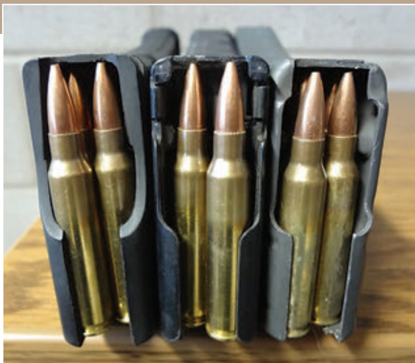
Two polymer magazines and a GI aluminum (right). Due to the thickness of the front wall on the far left magazine, the nose of the rounds catches on it. Close inspection reveals two impressions where they have been catching on it. Center polymer magazine had no issues and enough room for all types of 5.56mm ammunition.
