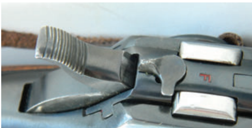
Hammer spur is nicely checkered and gives good purchase. Also visible are locking wedges and controversial placement of safety.
