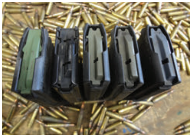
Almost every modern magazine manufacturer offers their own version of an anti-tilt follower with their magazines. Only old GI surplus magazines and some imitation knock-offs don't have it.
