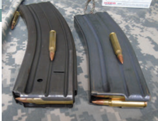
AR-180 magazines (left) are similar to their more familiar AR-15 counterparts save a small retention slot on the right side. AR-15 mags may be converted with some careful drilling and file work while still remaining usable in both rifles.
