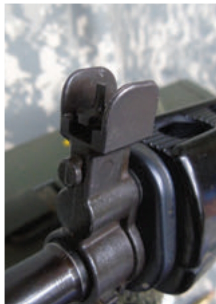
Front sight on AR-180 is fenced and adjustable for elevation.
