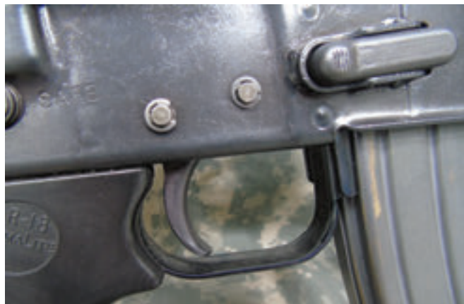
Like most of the rifle, magazine release is comprised of stamped steel component parts. Use of stampings made AR-180's design more amenable to less-developed societies than did all the forgings and millings required of the AR-15. Hammer and trigger pins are retained by simple industrial fasteners.
