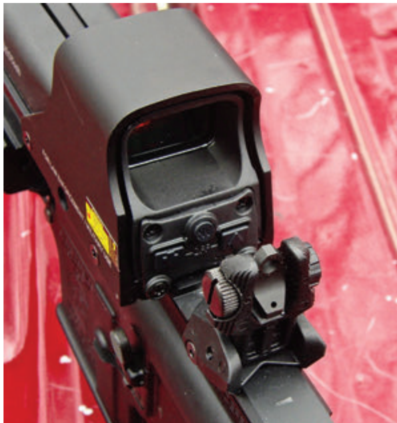
Above: Rear FRBS is mounted so that when flipped up, it allows use through the EOTech. It can be brought into action immediately if the holographic reticle fails.
