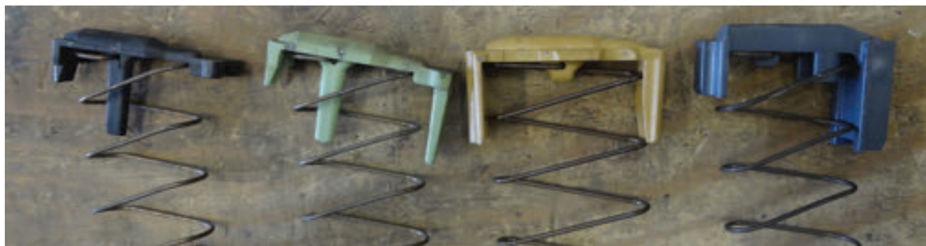
Above: Three followers from military-issued magazines and a Magpul Enhanced Self-Leveling Follower at far right. Compared to the old black follower, you can see the efforts to both lengthen and thicken parts of the follower to keep it from tilting in the magazine.
