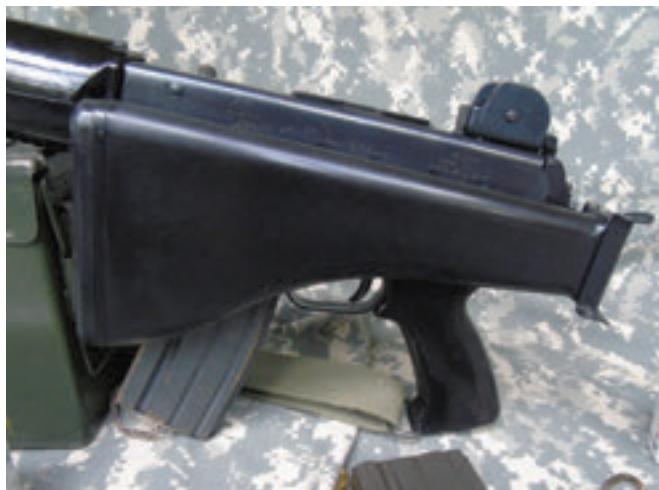
Recoil spring on the AR-180 is contained within the upper receiver assembly. This allows the rifle to incorporate a side-folding stock that makes it quite compact.
