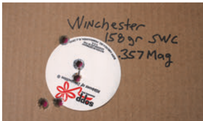
Winchester .357 Magnum 158-grain SWC loads produced this 25-yard group.
