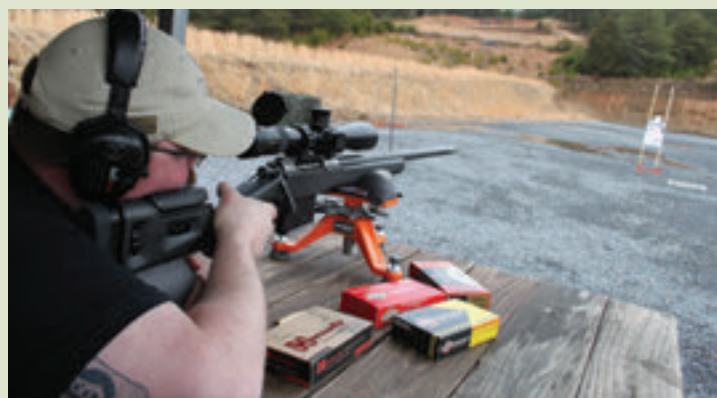
Initial bench testing was from a Champion pedestal rest and rear bags. Initial 25-yard paper sighting was followed by 100-yard groups.
