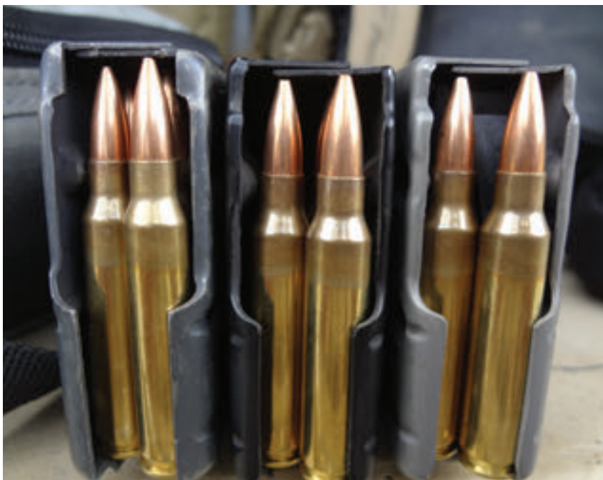
Three aluminum magazines. On the left, what the front folds of a magazine should look like, being evenly pressed together. The center and right magazines ... not so much. With the center magazine, due to the depth of the metal's fold into the inside of the magazine, rounds were dragging and getting caught up on it. This resulted in numerous malfunctions and made it an unusable magazine.
