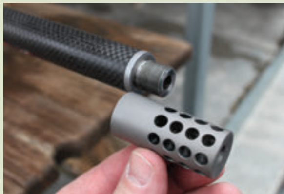
Radial titanium muzzle brake is threaded on Match carbon-fiber wrapped barrel via 5/8x28 threads.
