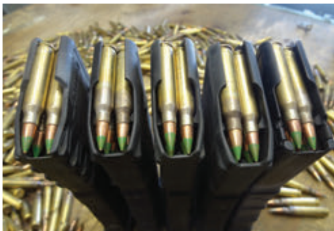
Five different polymer magazines. Polymer feed lips can wear out over time with hard use. Of the magazines pictured here, only the Lancer L5 Advanced Warfighter (far right) has metal feed lips.
