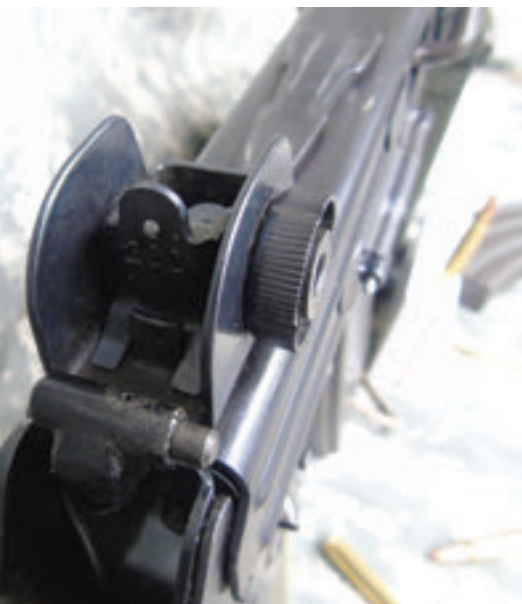
Sights on AR-180 are typical of its era. Flip rear peep sights are easily adjustable for windage.
