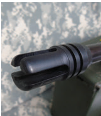
Flash suppressor on most AR-180s is similar to open-pronged version on original AR-15. While incrementally better at eliminating muzzle flash when compared to a closed sort, this design was prone to catch on vines and brush. Later AR-180s offered closed birdcage design.
