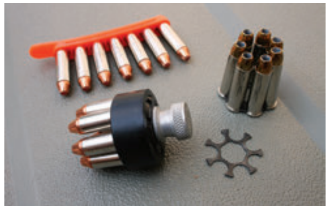
Tuff Strips combined with HKS seven-shot speedloaders give user great flexibility when combat loading. Full moon clips (right) are an all-or-nothing proposition.
