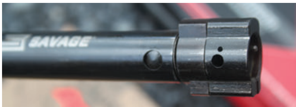
RIGHT: Savage bolt's floating bolt head. Lugs in front are independent of other set. Bolt handle has another gas baffle in front of it, at rear of bolt body.
