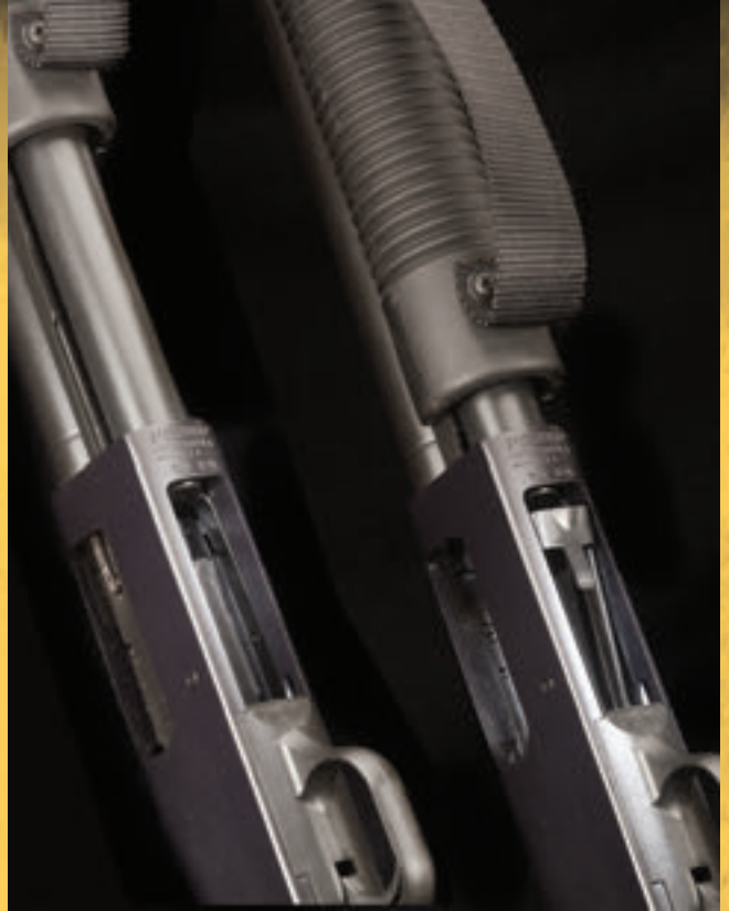
Well-designed anti-jam lifter is visible with action open (right). Twin action bars are not visible.
