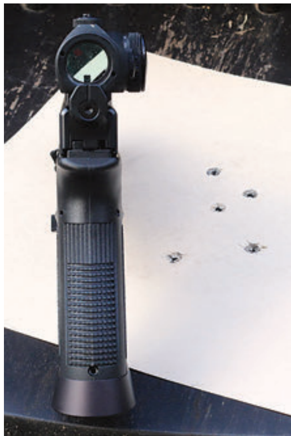
Five shots, each as fast as possible at seven yards with dot turned off and simply aiming through the Aimpoint's tube.
