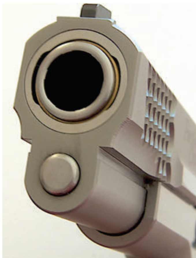
At the muzzle, Briley's excellent spherical barrel bushing, a critical component of 945's accuracy.
