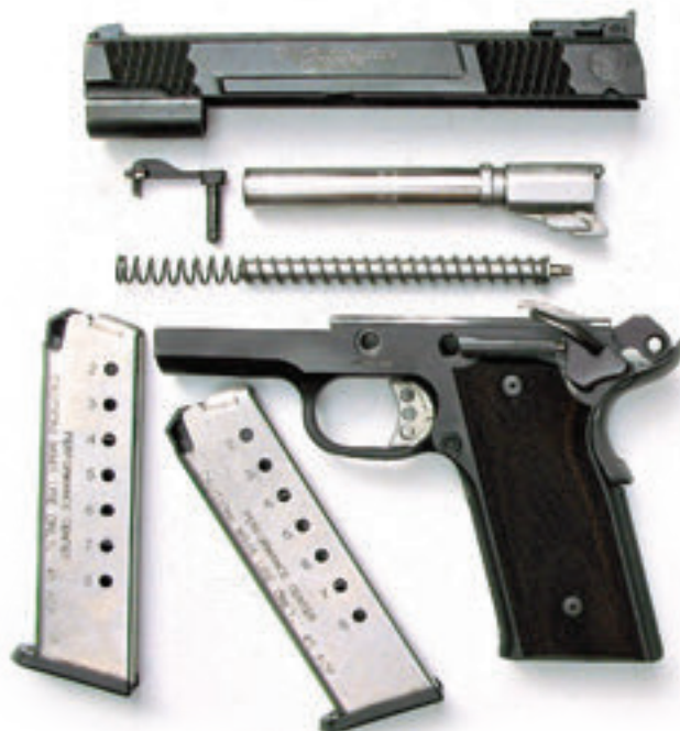
Author's 945 field-stripped shows linkless barrel and 14-pound recoil spring with guide rod that has its own internal spring. Magazines are eight round. Stocks are wood laminate. Hex screws were later changed to slotted screws.
