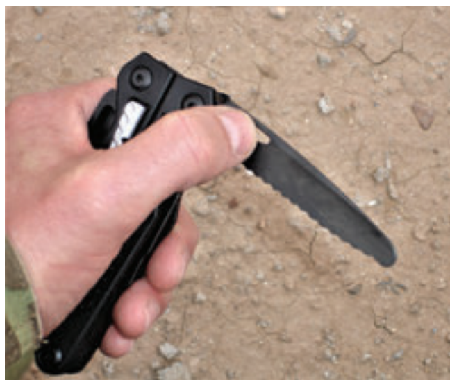
All blades and tools lock securely in place and are outside-accessible for one-handed employment.
