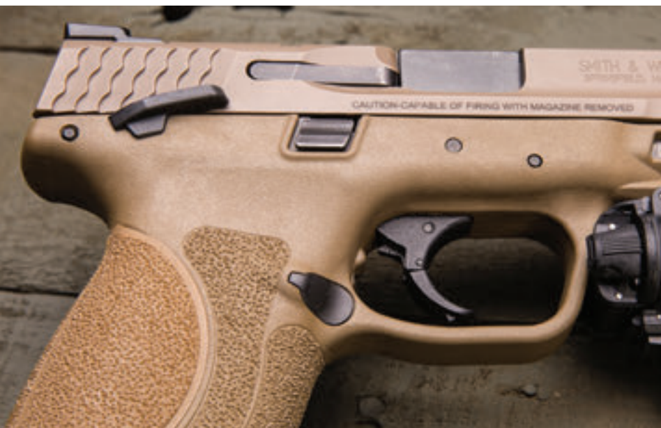
ABOVE: Right side shows ambidextrous safety and slide lock. Magazine release is reversible.
