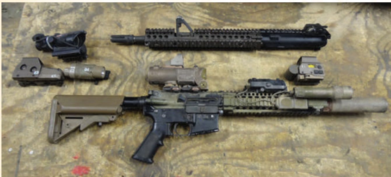
Current optic and light options available to SF soldiers. Left: EOTech SU-231, Trijicon ACOG, and old MX3 light. Mounted on MK18: SU-230 with EOTech MRDS, LA-5 laser, WMX200 light, and SureFire SOCOM suppressor. Just above LA-5 is latest CQB optic, SU-231A (EOTech EXPS3).
