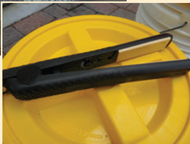
RIGHT: Standard electric hair straightener heat-seals Mylar bags. Look for a model with adjustable temperature control and experiment with different settings. Too high a temperature may damage Mylar bags and produce a faulty seal. Recommended sealing temperature is approximately 400 degrees.
