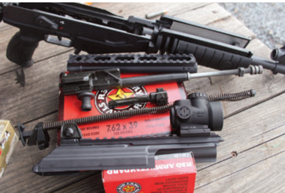
Galil ACE field stripped. Similarity to long-stroke piston AK is obvious.
