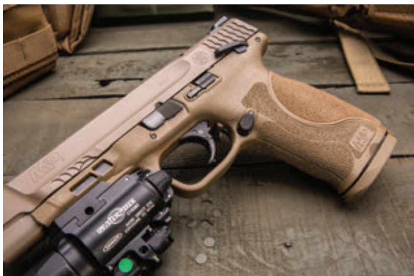
Left side of M2.0 shows mag release, safety, slide lock, and takedown lever. Only takedown lever is not reversible/ambidextrous.
