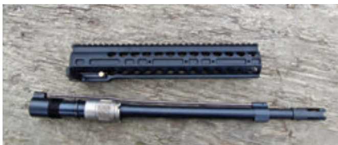
Handguard removed from barrel prior to assembling the rifle. Polymer thread protector on barrel has to be removed before assembly.
