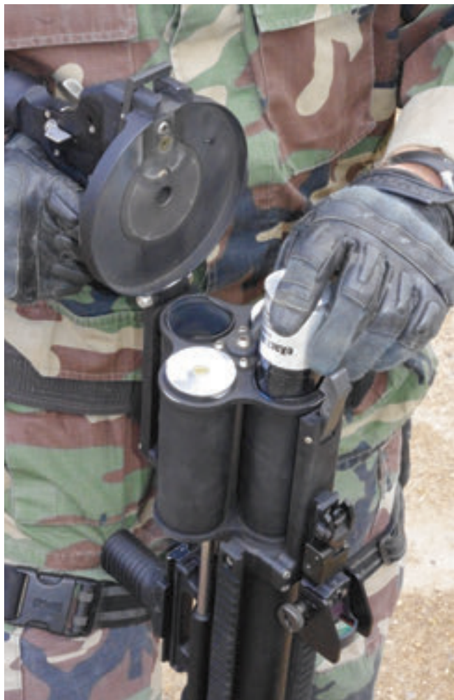
Tactical 4-Shot Launcher's circular magazine rotates around shaft that extends forward to forend. Grenadier demonstrates loading launcher while wearing gloves.
