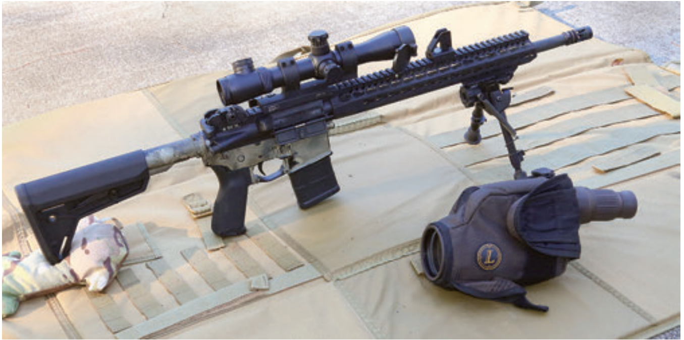
Test upper was a BCM mid-length 16-inch standard government profile barrel in a KMR A rail. Optic used was Leupold Mid Range Tactical 2.5-8X.
