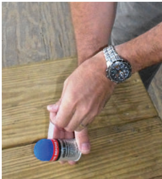
Projectiles are shipped in the "open port" configuration as a safety default, with a red tape strip that needs to be removed before use.
