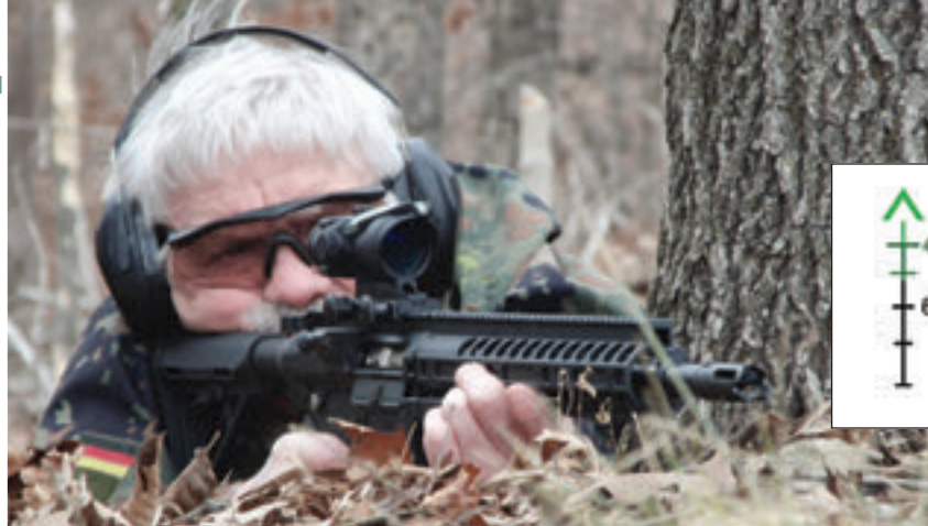
M762's 16-inch barrel allows good use of cover as well as keeping rifle compact for transport. INSET: Green chevron reticle used on ACOG employed in testing.
