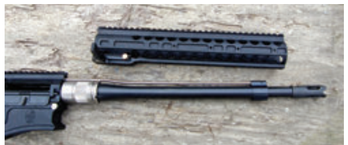
Barrel assembled to receiver and awaiting installation of handguard. Cross pin is pushed out and locking lever is up for installation of handguard.
