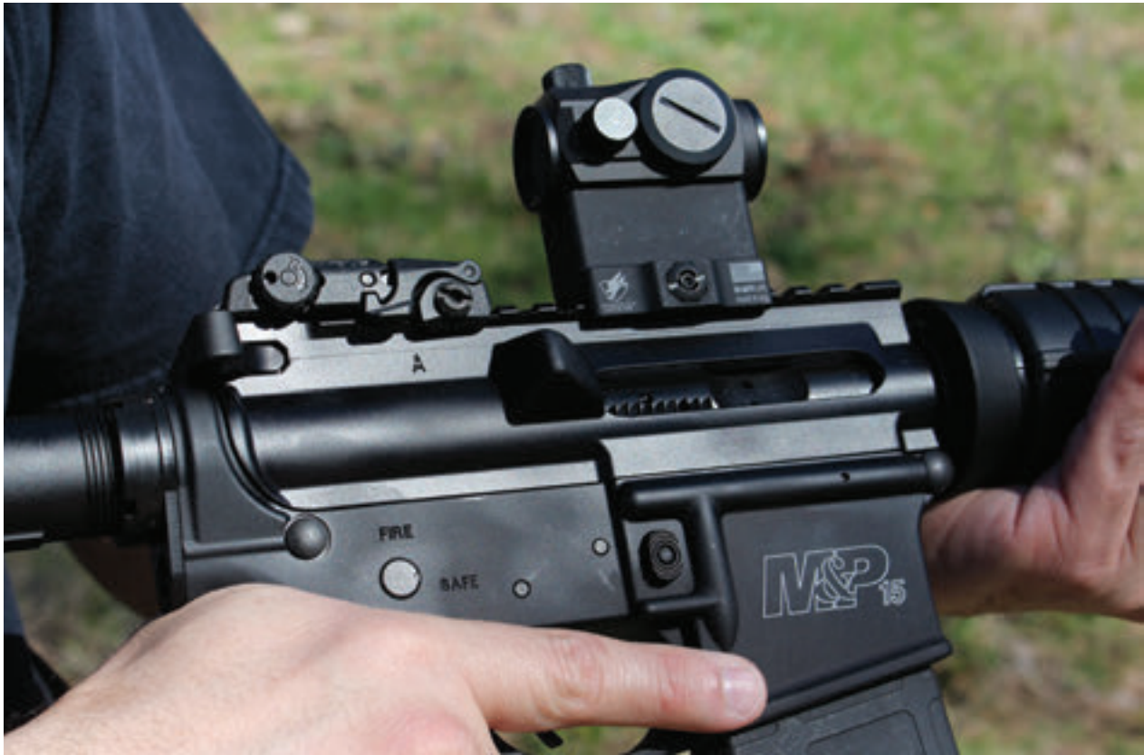
M&P 15 Sport drops the forward assist and dust cover.
