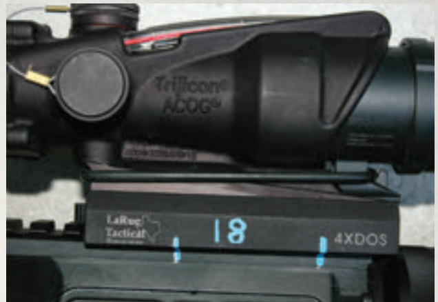
Make prominent paint marks so you can match the accessory to the carbine (in this case, a rack number) as well as witness marks on the mount and rail.
