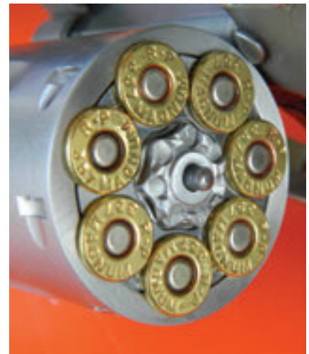
TK Custom machined author's S&W 686 Plus to accept moon clips.
