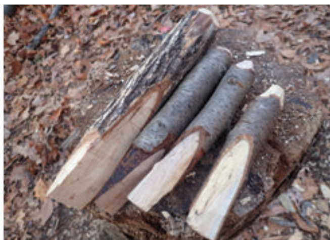
Wooden wedges made from dry hardwood. You need different sizes for splitting logs.
