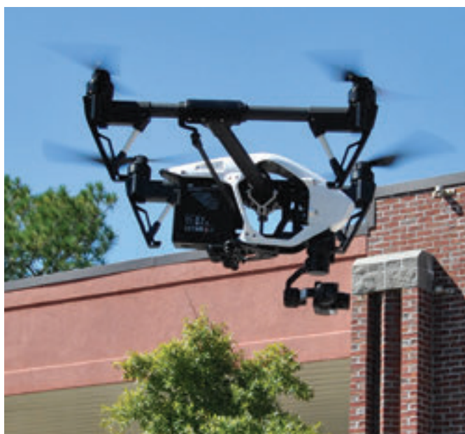
ABOVE: About seven feet off the deck, DJI Inspire 1 drone slows to a hover. This side view is a good vantage point from which to see the $2,000 drone's $13,000 FLIR camera.
