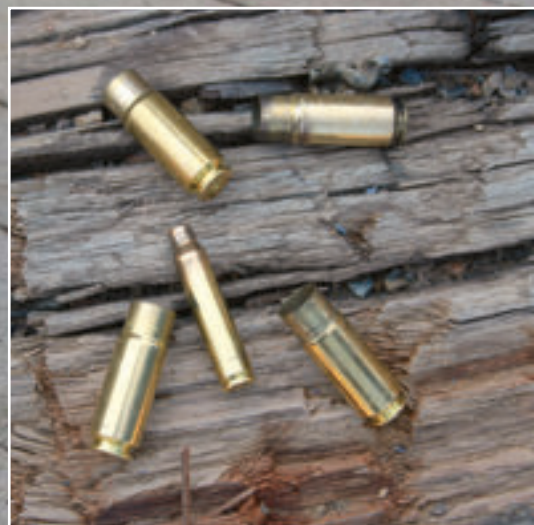
Empty .458 SOCOM brass surrounding 5.56mm casing. The .458 SOCOM is a lengthened .50 AE that is necked down to .458. Rim size is similar to .308 Winchester.
