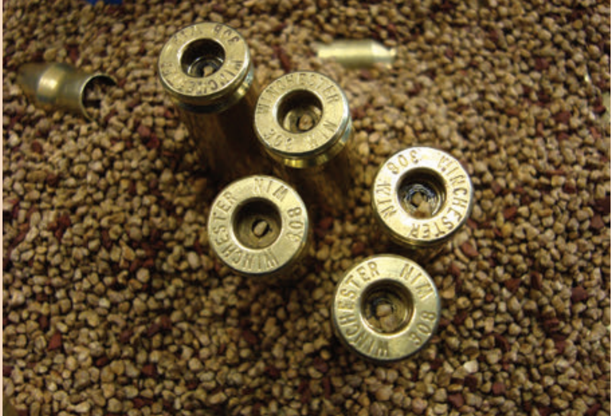
ABOVE: Cases are shiny clean after tumbling, but flash holes must be checked for stuck chunks of tumbling media (crushed walnut shells).
