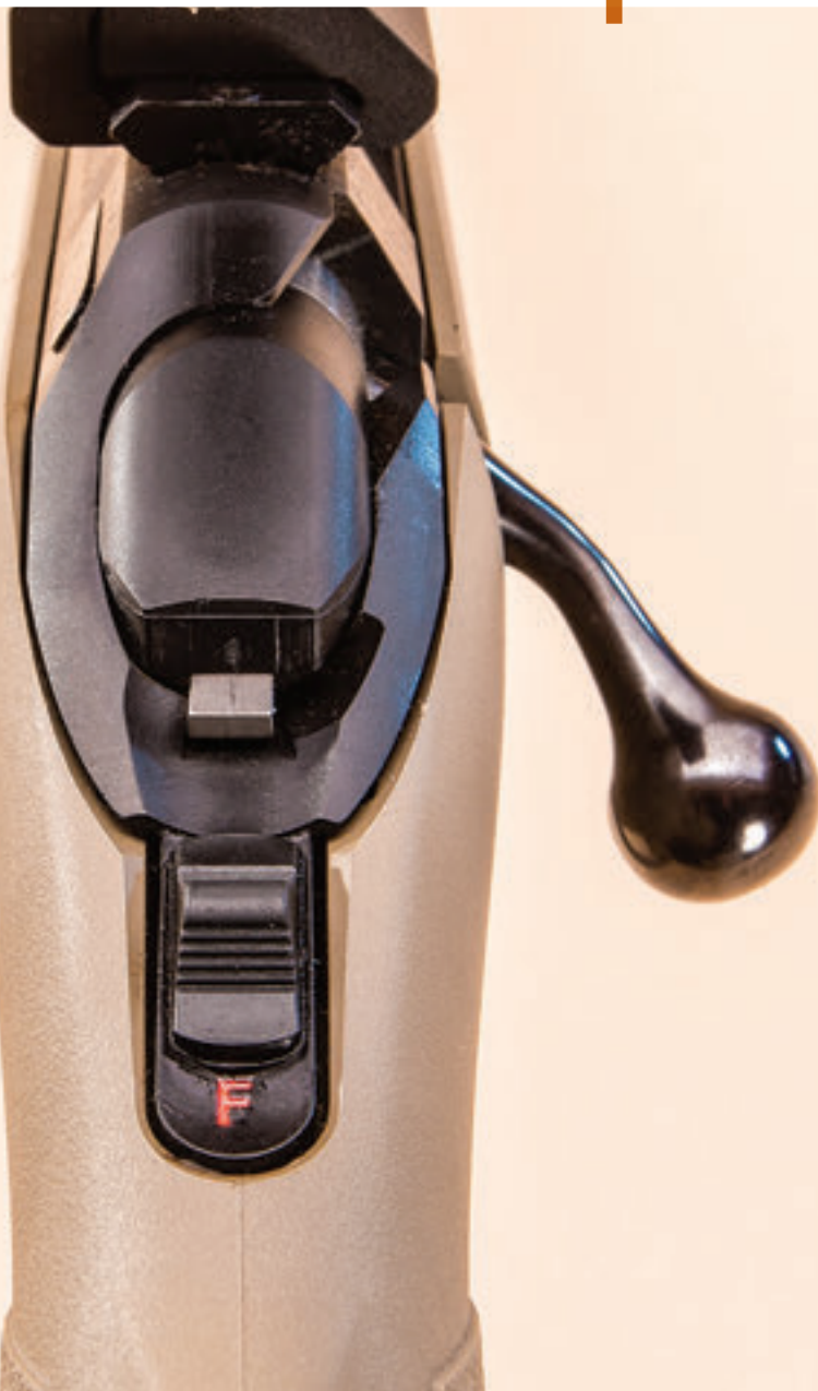
ABOVE: Indicator above safety is exposed when rifle is cocked.
