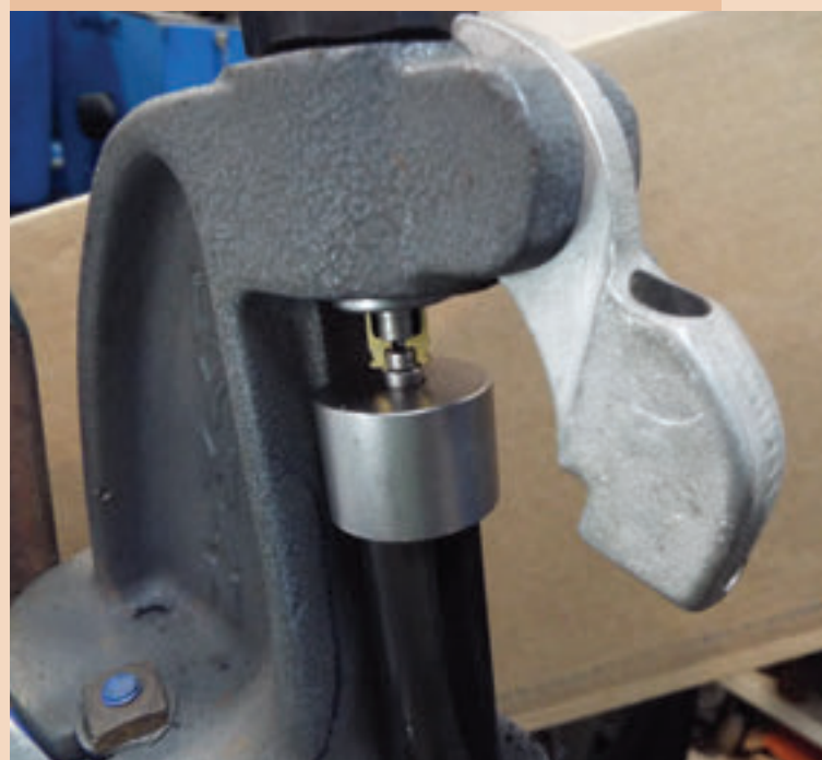
BELOW: Case preparation tedium ad nauseam . De-crimping military primer pockets cannot be skipped. Sectioned case shows top punch and swager with radiused step. Case web is squeezed via reloading press, crimp is reformed into a radius that eases insertion of new primer. No decrimp, no new primer insertion.
