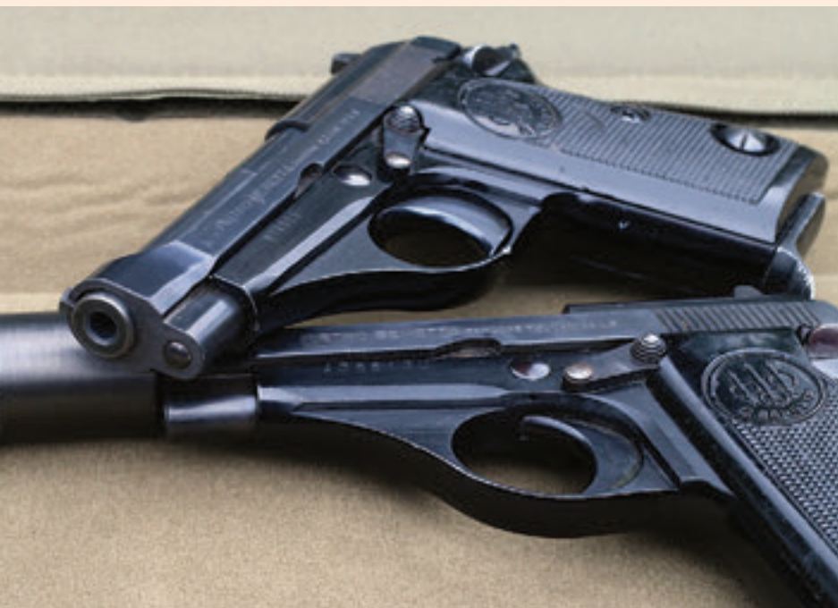
LEFT: Guerrilla Armament removed pipe and cut barrel back behind the threads to 3.2 inches on this surplus 71.
