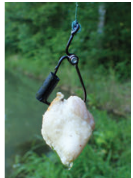
Baited hook would close when retrieved from the water. Hook would close easily when underwater, rendering both hooks useless.
