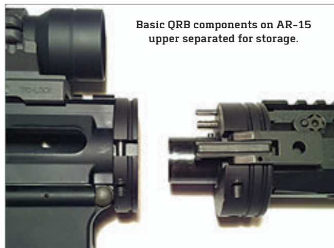
QRB receiver and barrel plate assemblies with special QRB nut, gas tube extension, stainless steel locating pin, and locking arms.
