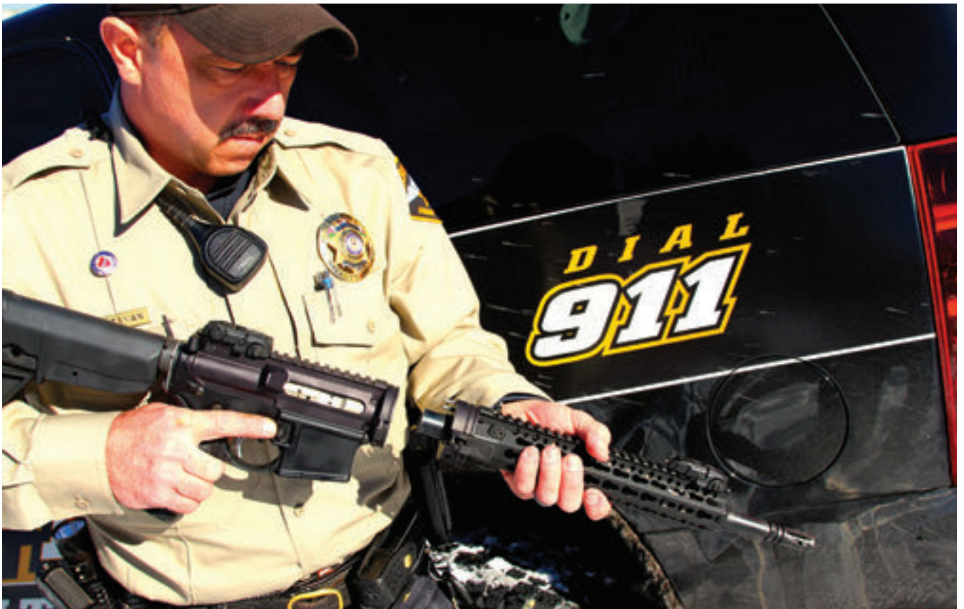
ABOVE: QRB receiver and barrel plate assemblies are attached to the receiver and handguard. Two-piece gas tube meets precisely when assembled.
