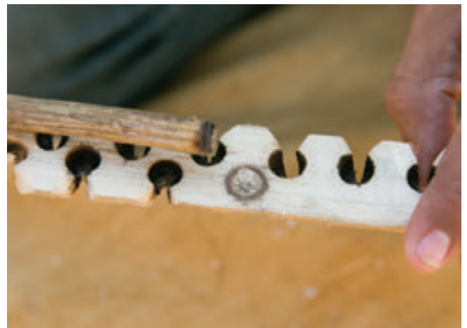
Creating a burn in. Before adding a V-notch, burn in the socket a little to know where the spindle will end up seating.
