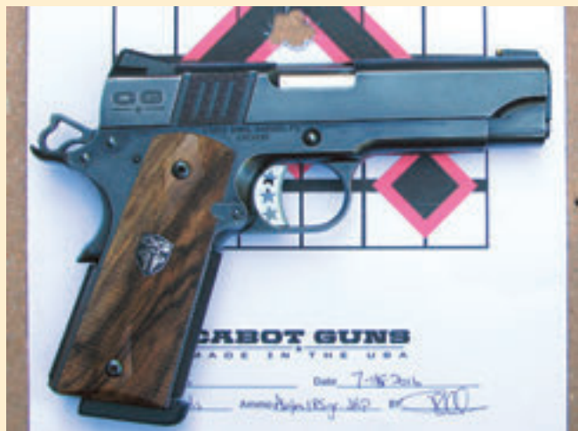
Cabot VCC with Trinity Strip slide checkering, semi-adjustable rear sight with gold-bead front, lowered and relieved ejection port, skeletonized hammer for faster lock time, billet steel grip safety/beavertail, and Turkish Walnut stocks. One-hole group was fired from Ransom Rest at 15 yards.
