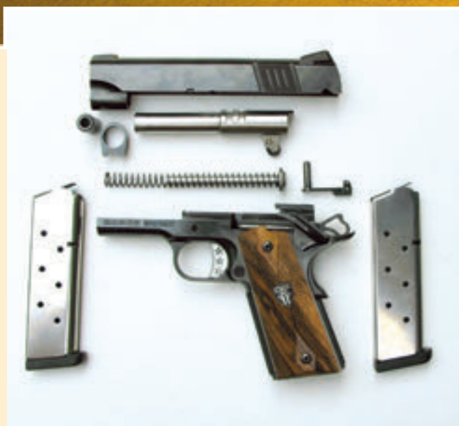
VCC field stripped. With exception of flat wire spring, pistol and parts are mostly forged from billet steel. Receiver rails are full-sized 1911 pistol for Full Cycle Technology and timing. Button-rifled and crown-cut barrel is hand fitted.
