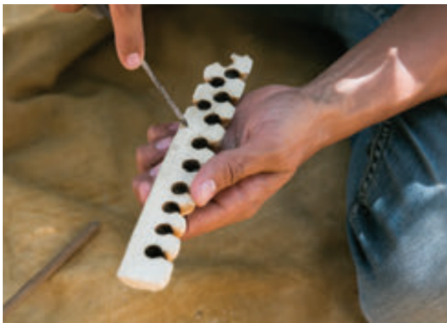
Drilling the socket for a place for the spindle to seat.
