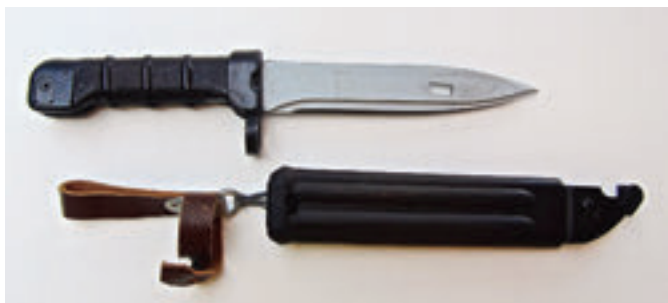
ABOVE: Russian AK-74 bayonet has spear-point blade and more ergonomic handle.
