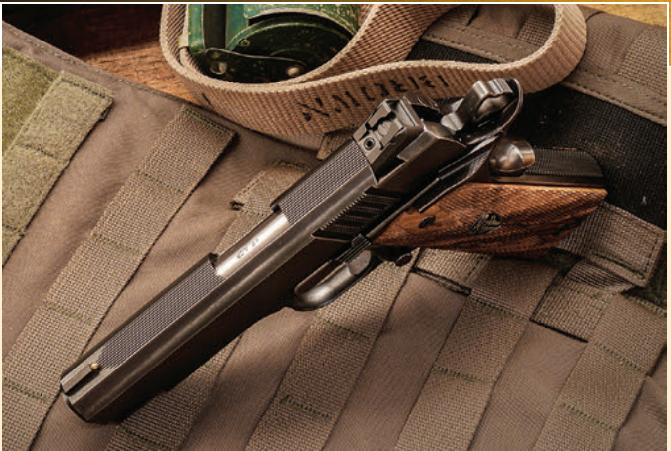
Top of slide has arrow-pattern serrations that cut glare and draw eye to front sight, whose gold bead is evident. Novak rear aperture is adjustable for elevation.
