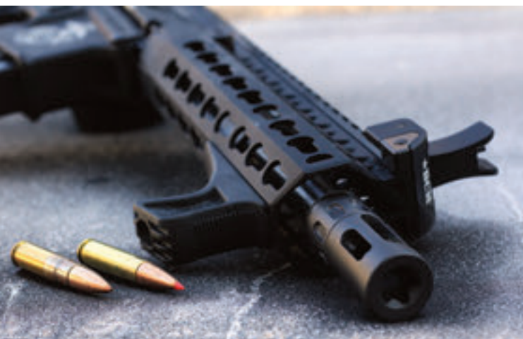
ABOVE: BCM Recce-9 KMR-A Pistol in .300 AAC Blackout hits like a rifle, with standard .308-caliber projectiles stuffed into a necked-up 5.56mm length case.
