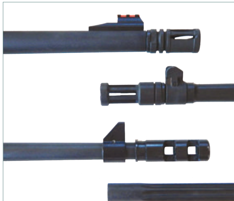
Muzzle devices, or lack thereof. Top to bottom: Mossberg, Ruger, Savage, and Steyr.
