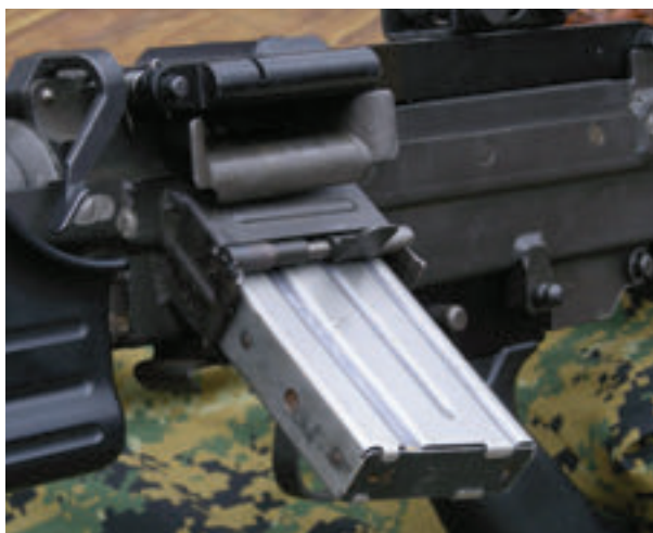
Although capability exists to use STANAG magazines with the M249, it is not a desirable option.
