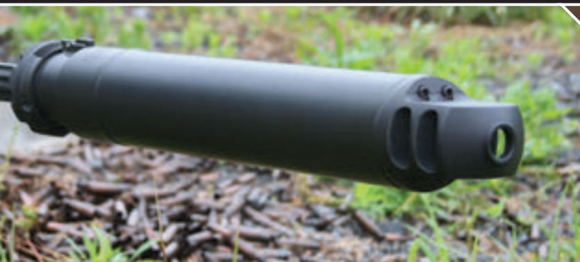
Barrett QDL Suppressor enhances M107A1's performance by reducing muzzle signature when fired.
