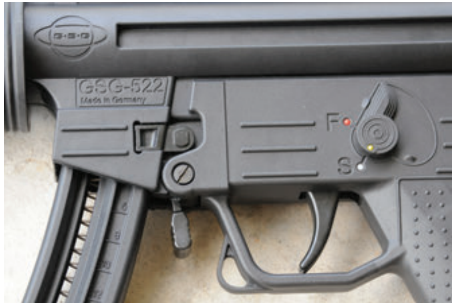
Ambidextrous safety selectors on GSG5 have high angles that are difficult to actuate with the thumb.
