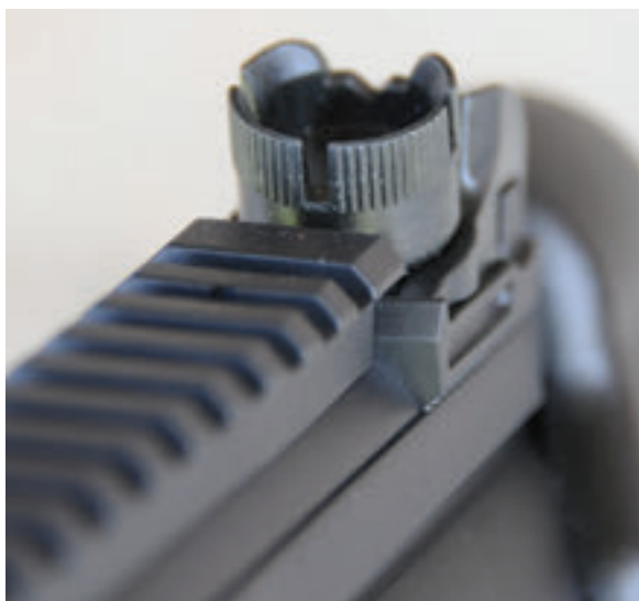
GSG rear sight has no vertical limit for frame reference on the front sight. But CQB notch is an excellent configuration for short-range shooting.
