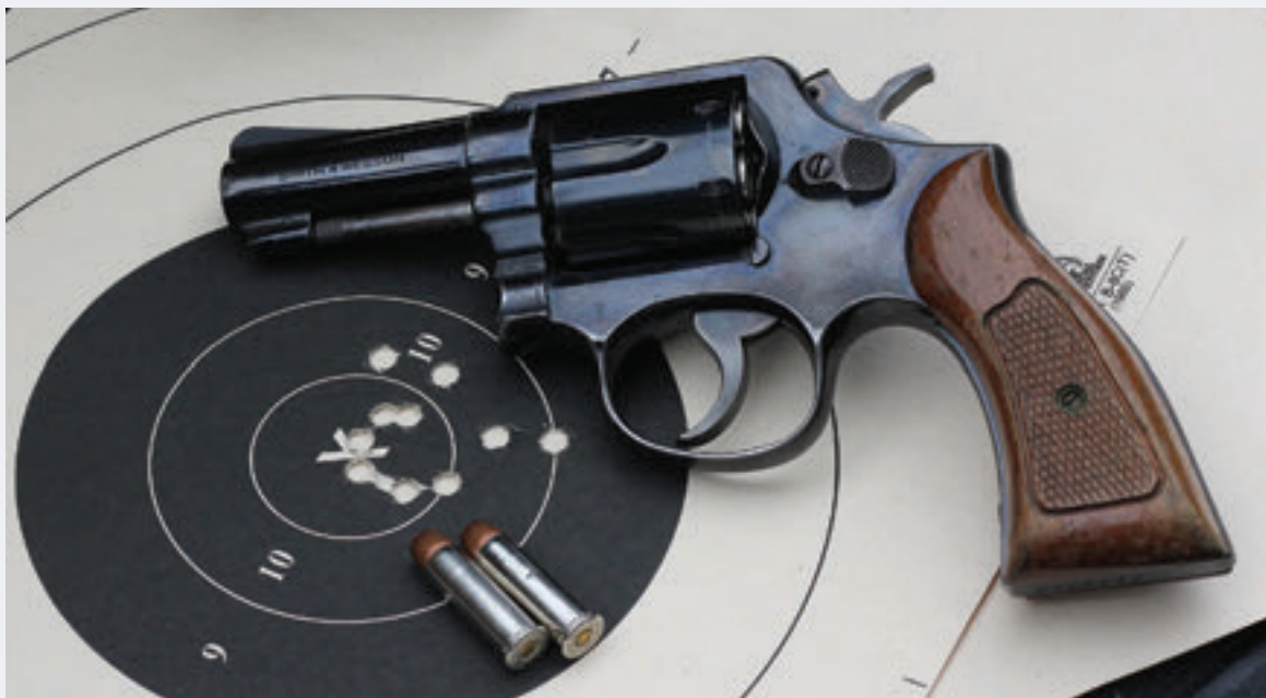
Model 10 was bragging-rights accurate with Winchester Ranger JHPs, as this 1.7-inch group from 25 yards shows.
