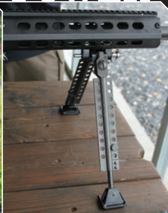
Barrett has incorporated titanium in M107A1's bipod legs, leaving no stone unturned in their quest to reduce weight while increasing strength.
