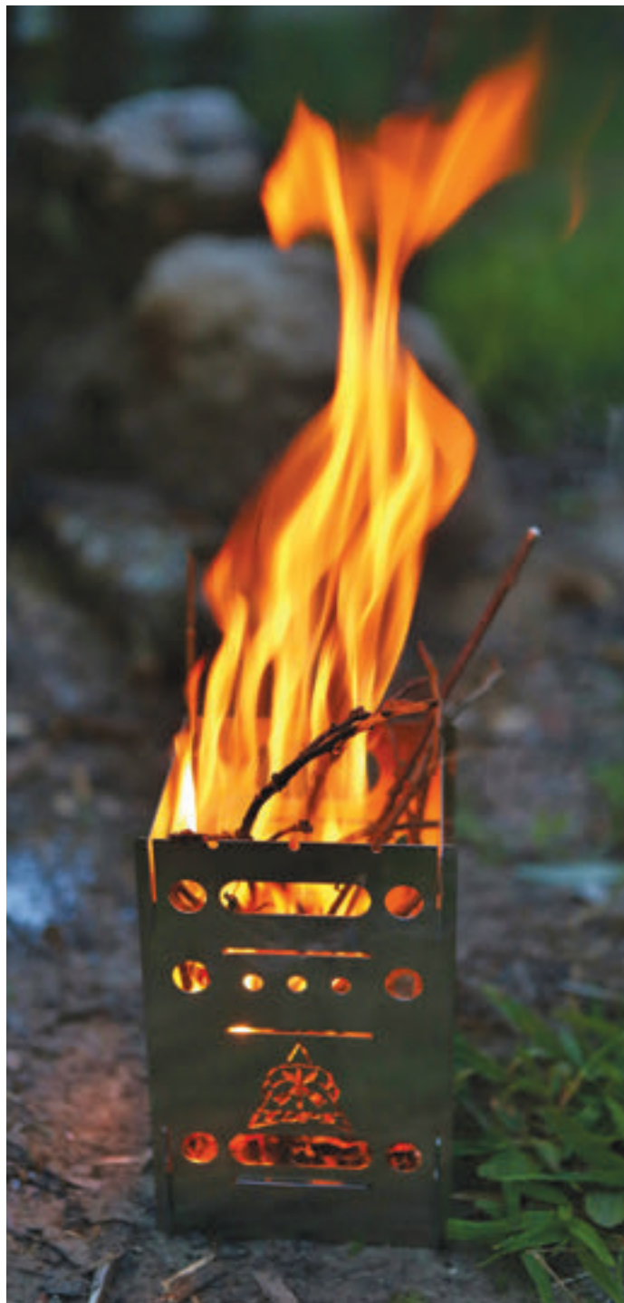
As a standalone wood-burning fire, author used this for a small controlled survival fire. Fuel can be fed into the stove from the top. Damp wood can be dried by placing it across the top.
