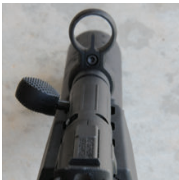
HK sight picture is traditional diopter configuration. Author found this configuration faster and more user friendly than GSG's square-framed sights.
