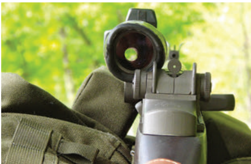
View from rear of offset scope, which allowed M1D to still be loaded with eight-round clips.
