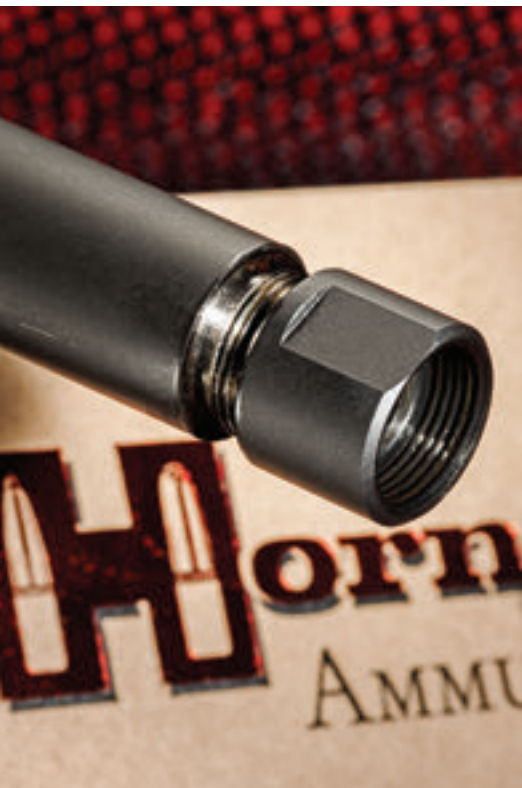
Muzzle features 5/8x24 threads for attaching a suppressor, and comes with a thread protector.
