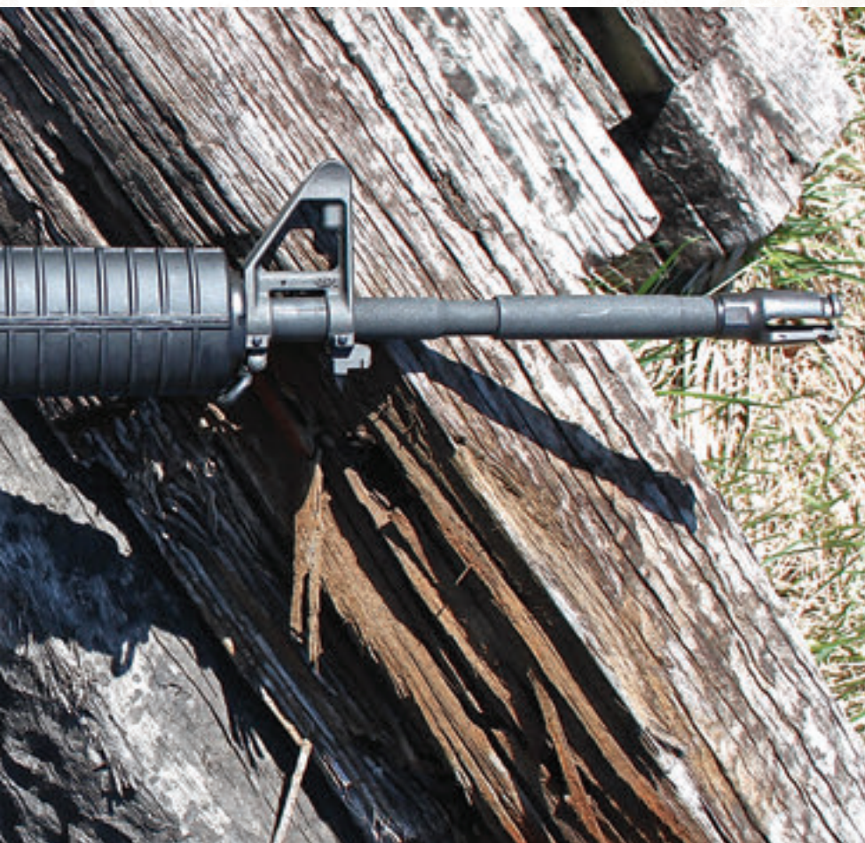
Standard A2 flash hider was replaced with Valmet-pattern VAL-76 three-prong flash hider.
