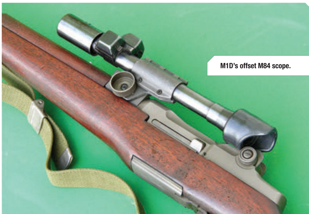
View from rear of offset scope, which allowed M1D to still be loaded with eight-round clips.
