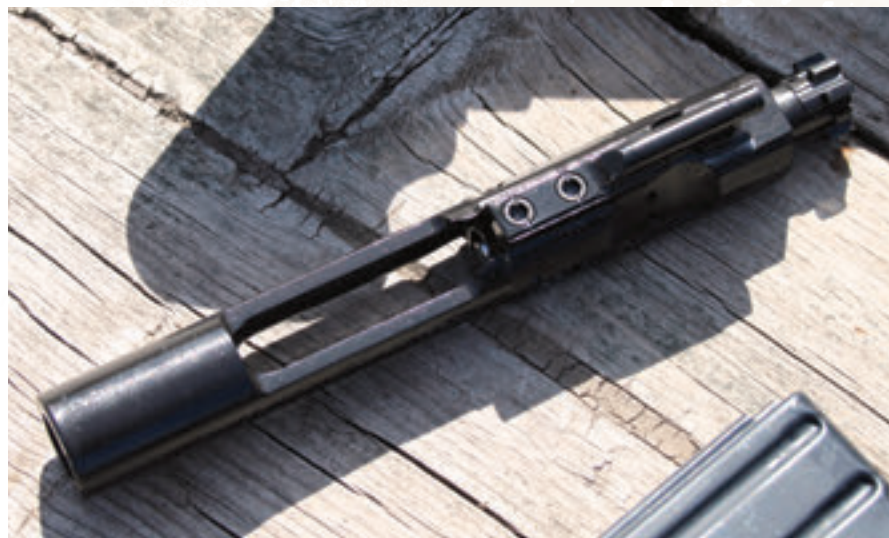
Above: Carrier key was properly staked.
