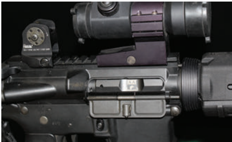
Adams Arms gas piston bolt carrier and system in the AR.
