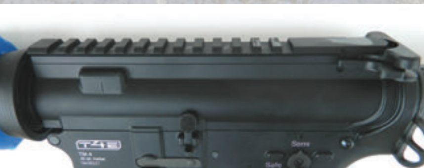
Top Picatinny rail is "T" marked to allow repeatable zero of optics.
