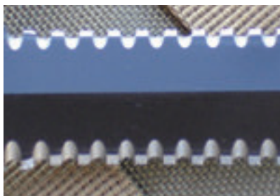
Double serrations were added to Gerber Mark II in the 1970s. When Gerber reintroduced Mark II in 2008, serrations were changed from scalloped saw teeth to flat chisel shaped.
