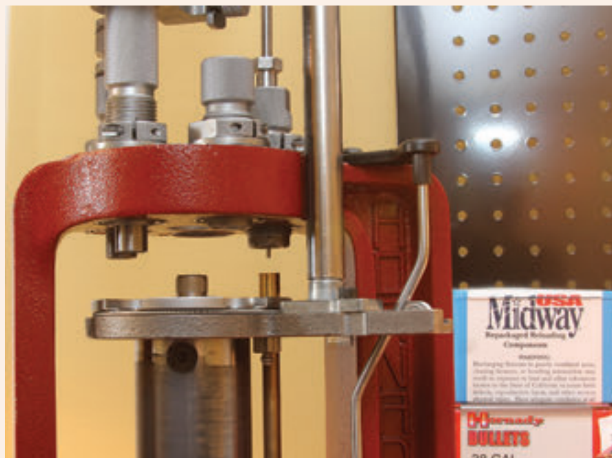
Author battled resizing die for the first 100 rounds until getting it set correctly. Lesson learned: if it's not working smoothly, it isn't set correctly.
