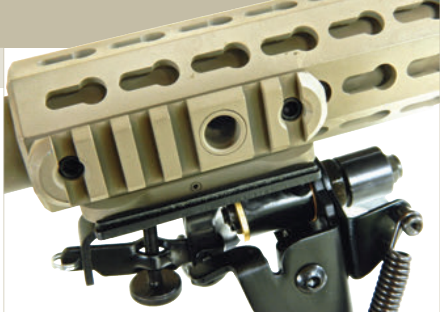
One rail section has a QD sling socket, while another has a stud for attaching a bipod.
