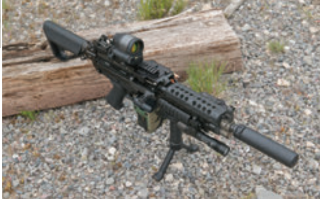
Using SureFire SOCOM Mini-762, SAW K remains compact. It weighs in at almost four pounds less than a standard MK 46.
