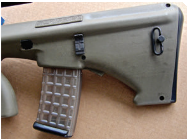
AUG's cross-bolt safety, bolt release lever, and magazine release button/lever, plus very durable 30-round polymer magazine.
