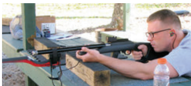
Chronographing unsuppressed rounds with MagnetoSpeed V3 Ballistic Chronograph and See All Open Sight.
