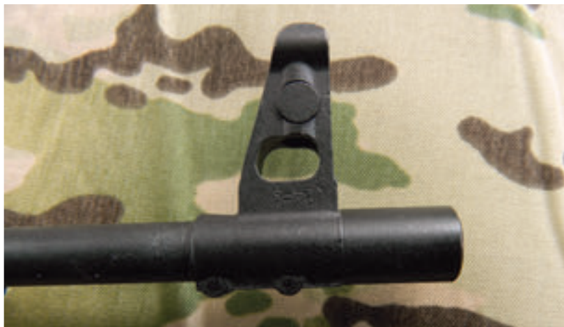
Above: MR has no muzzle device and barrel is not threaded for one.
