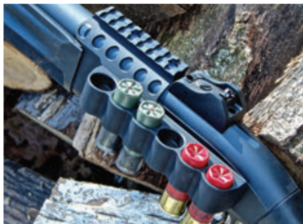
Above: Left side of 1301 shows Mesa Tactical SureShell shotshell carrier and rail. Inset: Ghost ring sight with white dots is very useful for low-light aiming.
