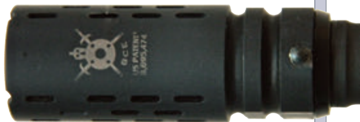
Permanently attached BattleComp 1.5 compensator brought 14.5-inch barrel up to 16-inch legal requirement.
