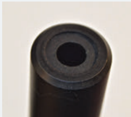
Left: Recessed step-type muzzle crown provides good protection for critical last part of barrel's rifling.
