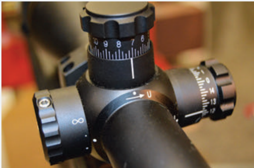
Turret knobs of Leupold Mk4 scope. Clicks are sharp and distinct, even with gloves.
