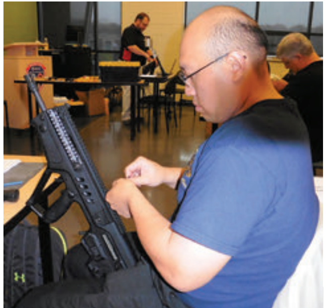
Student reinstalls cocking handle guide and Picatinny rail.
