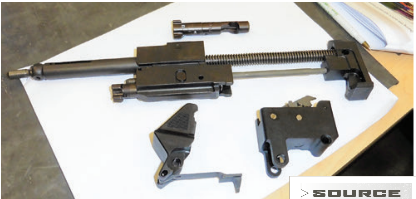
Converting 5.56mm to 9x19mm SMG with bolt carrier and firing group.
