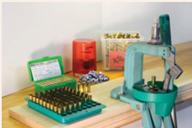
Expensive high-tech tooling is not required to build quality ammunition. Proven old tools like the RCBS Rock Chucker press and Lee carbide dies produce exceptional handloads.
