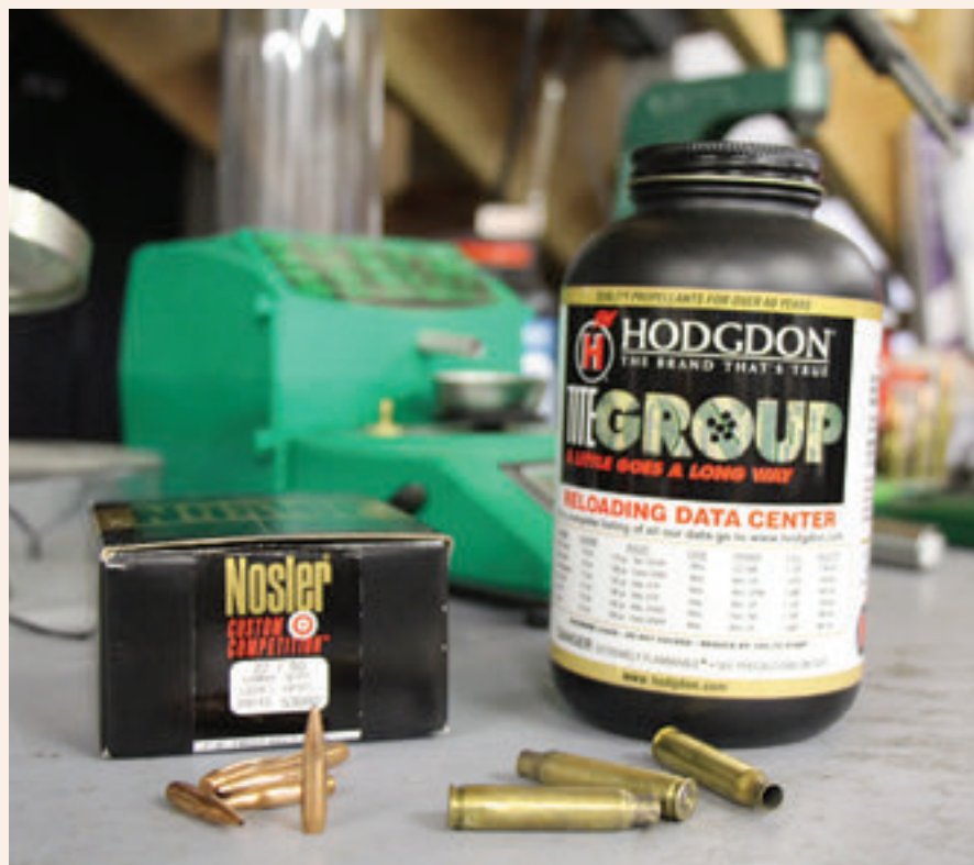
Nosler 80-grain bullet and Titegroup performed best with subsonic velocities but would not work the AR action.
