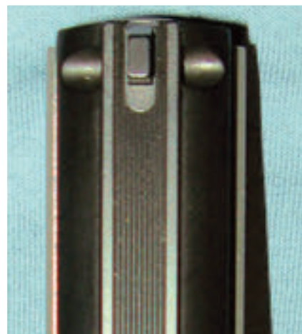
Dorsal side of slide with striations that run from rear to front sight. Striations draw shooter's eyes to the front sight.
